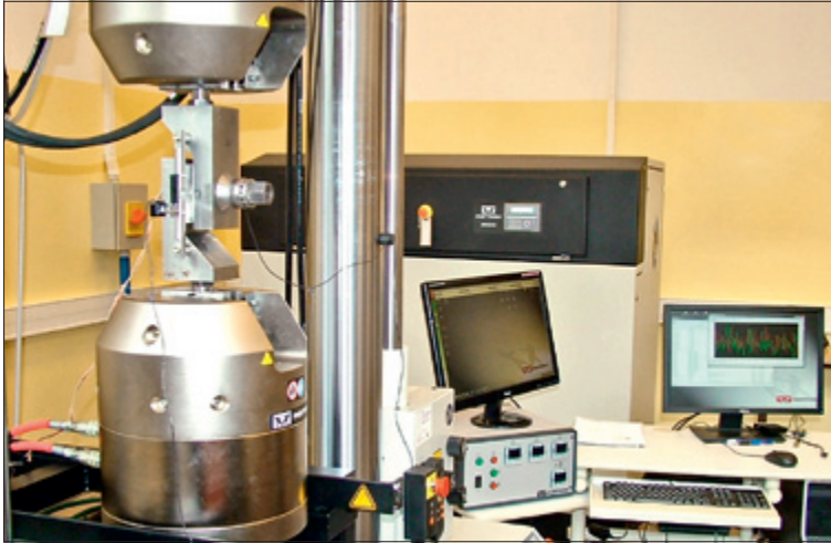
Fig. 8.72. Execution of the tests on the bolt joint with steel chock by using 8850 INSTRON strength testing machine
