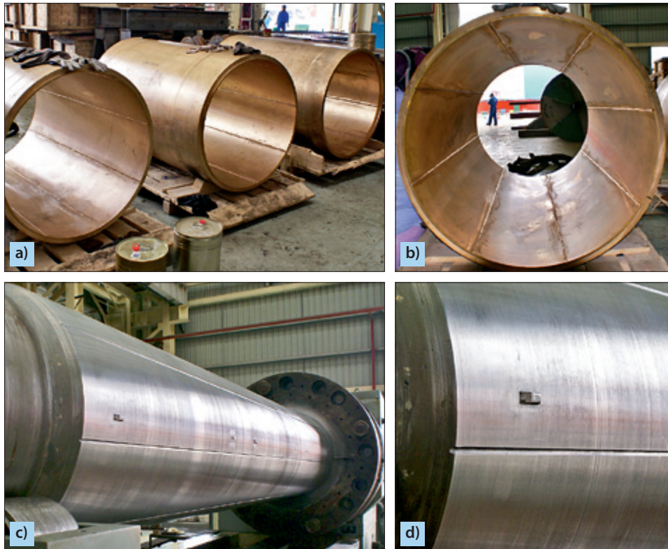
Fig. 6.15. Segments of the bearing liner and shaft with cut grooves and welded distance elements
