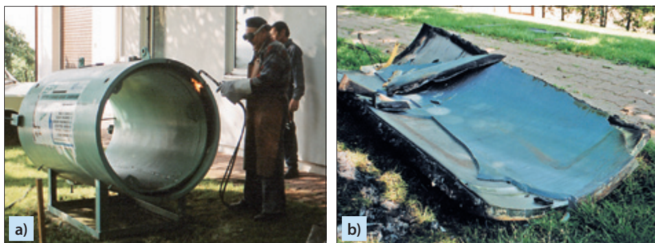
Fig. 8.33. Stern tube assembly model (frame tube and propeller shaft stern tube with EPY compound layer in between) during its dismantling: a) gas cutting the outer pipe; b) upper part of the outer pipe, cut-out together with EPY compound layer
