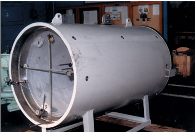
Fig. 8.30. The model of the assembled system of propeller shaft stern tube and frame tube, fitted with sensors for measuring relative displacements of joined elements
