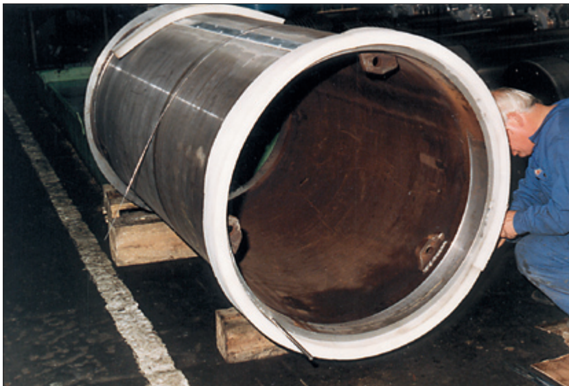
Fig. 8.27. The model of propeller shaft (bearing) stern tube (inner pipe)
