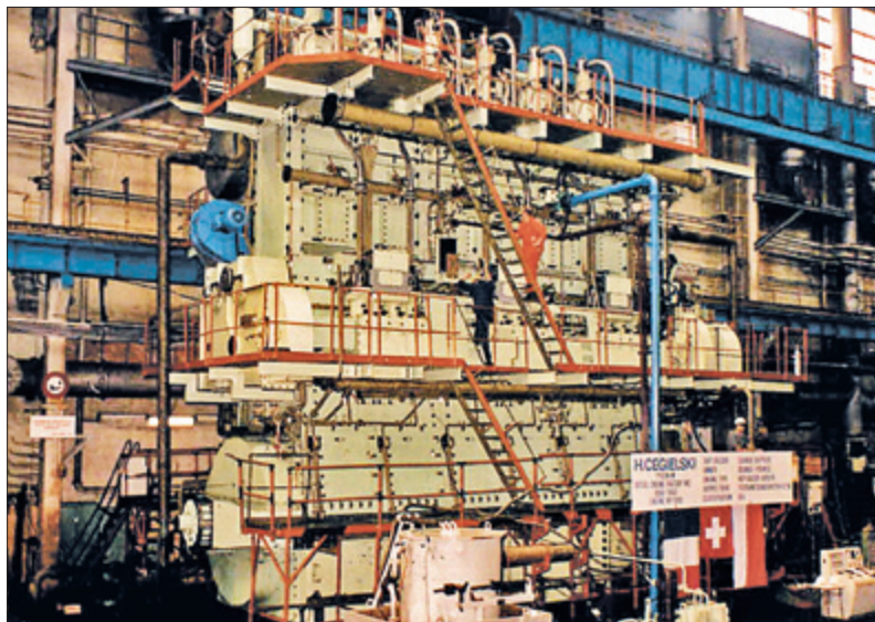
Fig. 6.1. 6RTA76 HCP-Sulzer main propulsion engine (on test stand)
