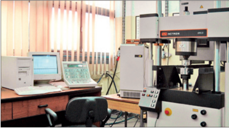
Fig. 7.12. Test stand for determination of mechanical characteristics during compression test at various strain rates
