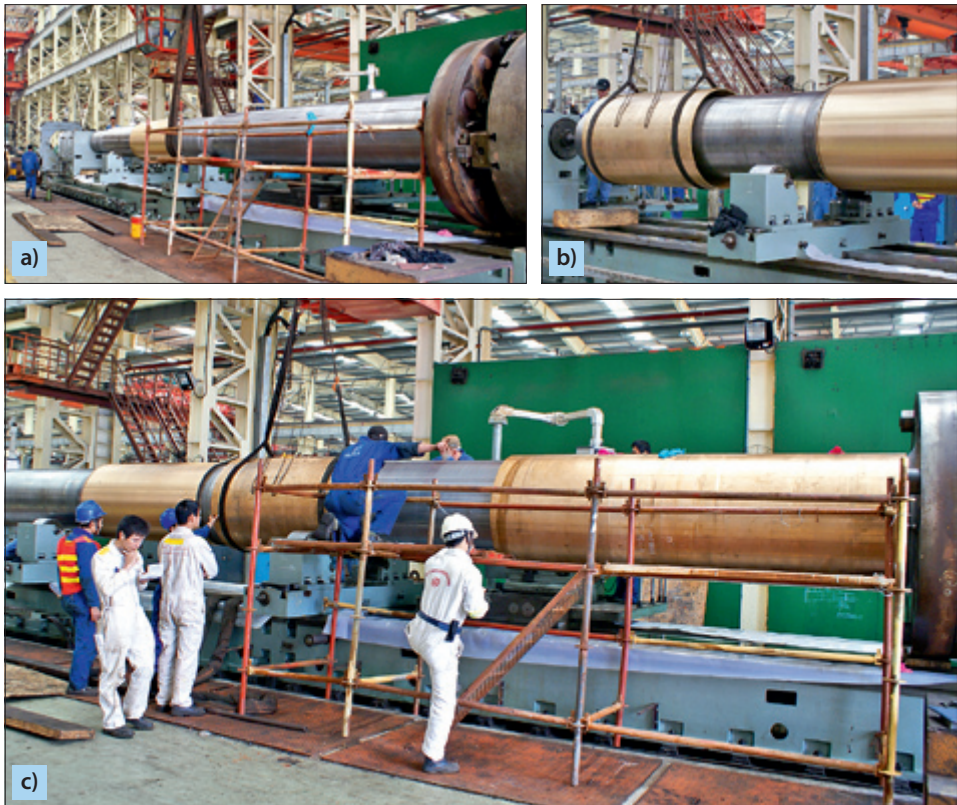
Fig. 6.16. Run of the inserting operation of particular segments of bearing liner onto shaft
