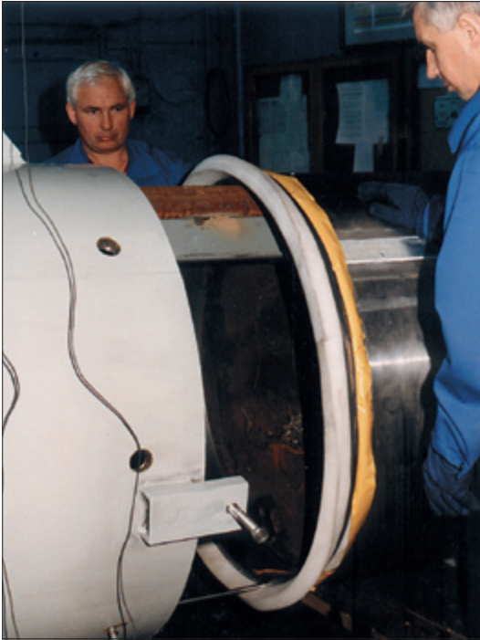
Fig. 8.29. Fore packing made of polyurethane foam and steel band (before mounting)
