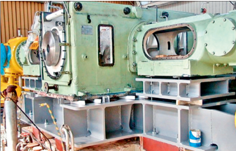
Fig. 6.47. The aligning of particular compressor components by means of adjusting screws and wedges
