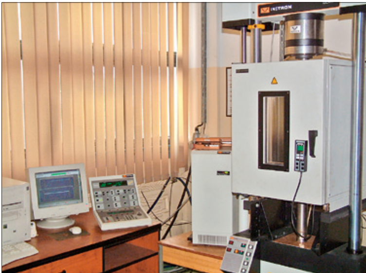
Fig. 7.25. Test stand for determining compound deformation characteristics under constant compression at increasing temperature
