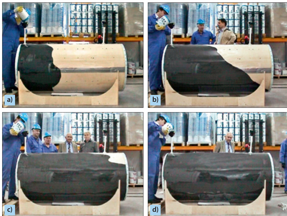
Fig. 6.14. Model tests on run and time of filling the pouring gap between shaft and liner with liquid EPY compound
